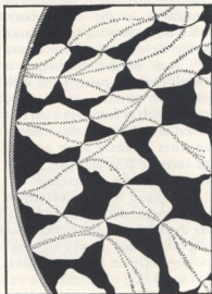
FIG. 3. Carbon grains in a transmitter magnified about fifty times each way. When the diaphragm is bent in (at left), the grains are closely packed together and many electrons can pass through. But when the diaphragm springs back (at right), the grains are loosely packed and fewer electrons can pass from grain to grain through the chamber.
