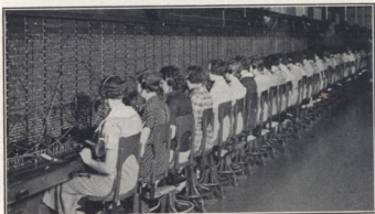
The multiple switchboard in your telephone city may have up to 10,000 connected telephones, and your operator can connect you with any one of them.
