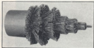
Here is a section of an aerial telephone cable fanned out to show the paper-insulated wires.
